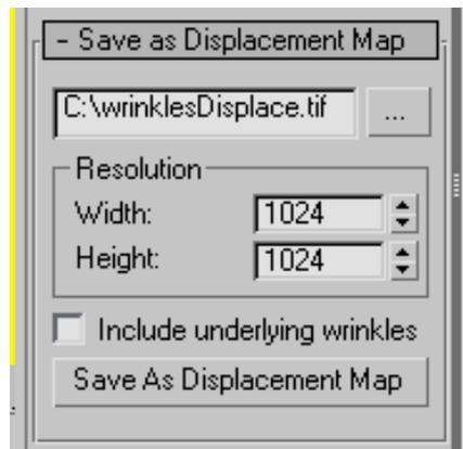
This rollout serves for saving wrinkles as displacement map for further use on low poly geometry.
